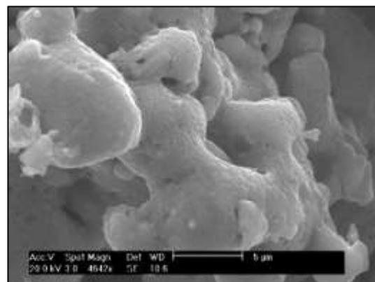
**Figure 2: Micrograph of 45S5 bioglass mixed with naphthalene pore-creator**
