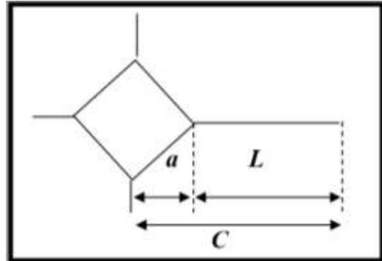
Figure 1. Crack measurement using Vickers indentation
