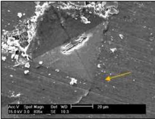
**Figure 3: SEM micrograph showing initiated crack by Vickers indentation method.** *Physical Properties*
