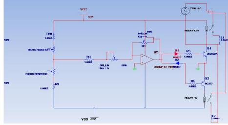
Figure (6) show circuit diagram for tracking system.
