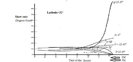
Figure (2) Variation in the rate at which the solar azimuth and altitude angles change for three representative days. The latitude is 32 degrees for this example.
