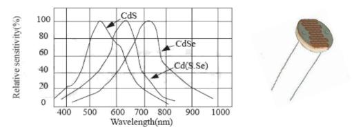
Figure(3) The Relative sensitivity CdS, CdSe, Cd (S.Se) with wave length [10].
