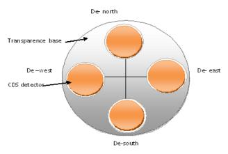
Figure (4) Distribution of CdS detector on a sensor head
