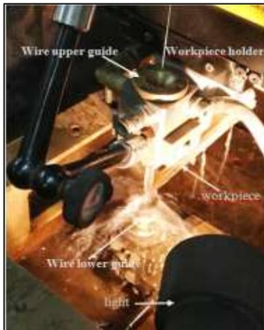
Figure 4: Electro wire cut machine
