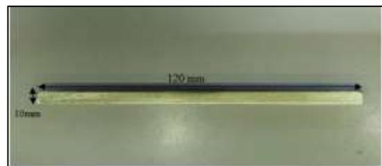
Figure 6: shows the workpiece before machining
