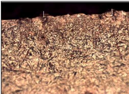
Figure 10 & 11: Cross section micrograph HAZ & WLT at TON=110
