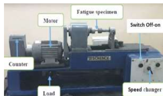
Figure 2: Fatigue rotating bending machine (SCHENCK PUNN).
