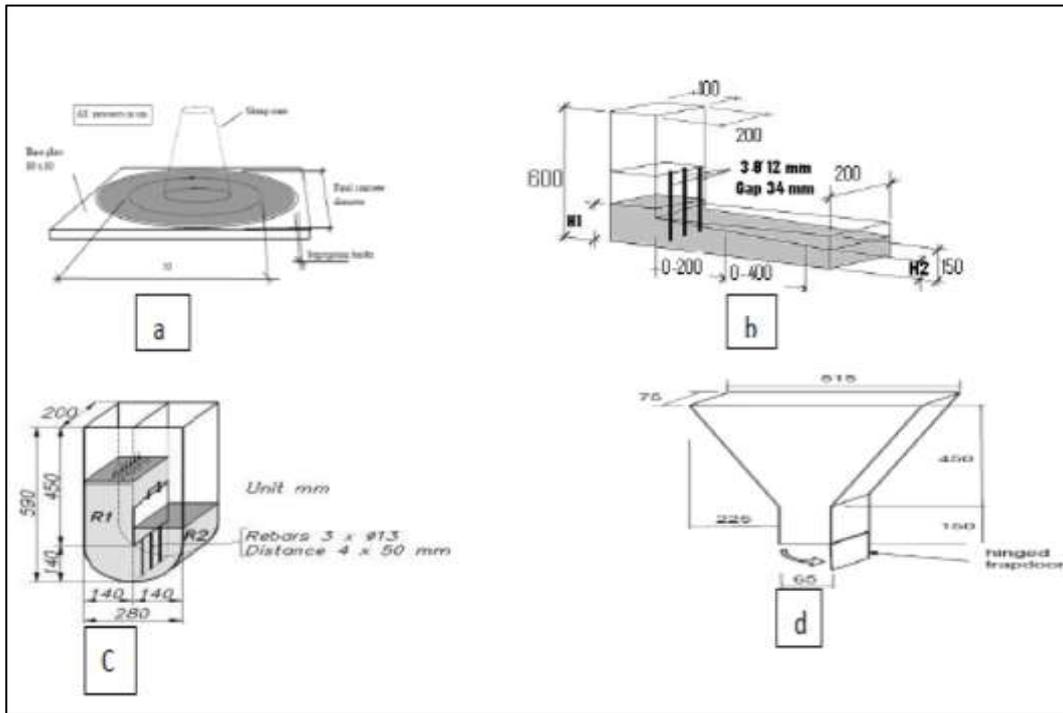
Figure 1. a) V-funnel b) L-box c) U box test set up Hardened State Tests
