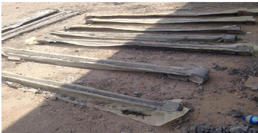
Plat(4): Specimens For Drying Shrinkage Cracks.
