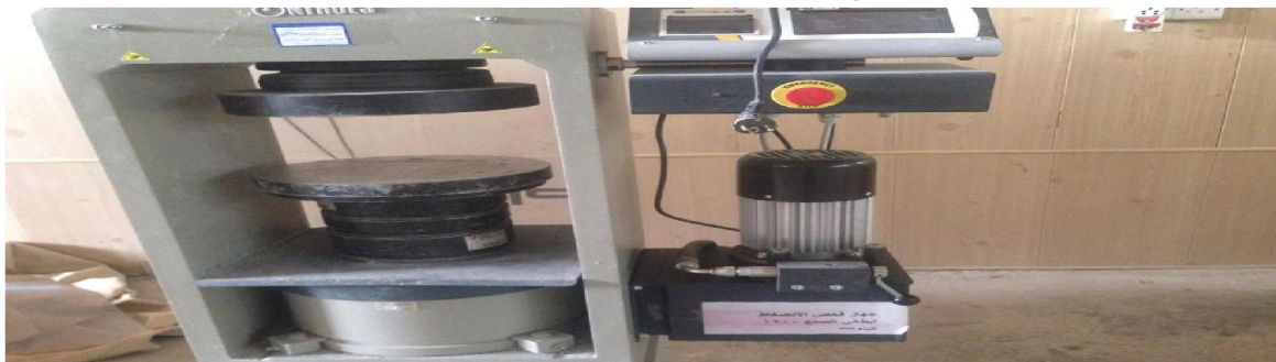
plat ( 7 ) : Compressive Strength Testing Machine.
