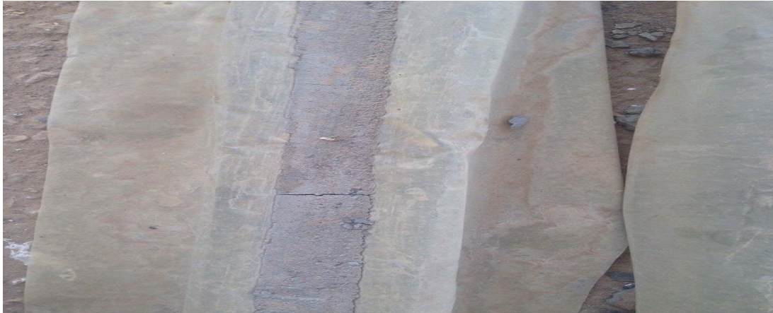
Plat(8):- specimen for Drying shrinkage cracks for mix (MD0.4%) .
