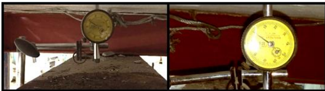
Figure (5): Dial Gauge Used to Measuring Deflection.
