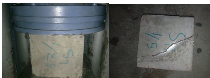
Plate (2): compressive strength test
