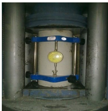
Plate (3) modulus of elasticity test
