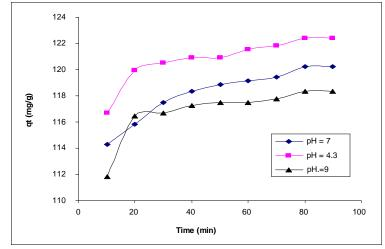
Figure (1): Effect of contact time of the removal of 6MBT- BN dye of various pHs.
