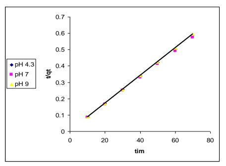
Figure (5): The plot of t/qt versus time at different pHs for 6MBT-ßN dye
