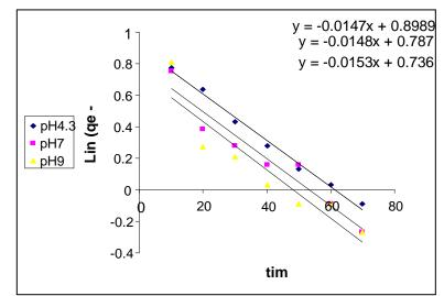
Figure (4): The plot of log (qe-qt) versus time at different pHs for: 6MBT-BN dye
