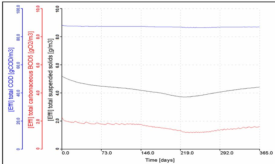
**Fig. 8: Simulation results of COD, BOD<sub>5</sub> and TSS in effluent under yearly variation of Wastewater temperature at average influent flowrate**
