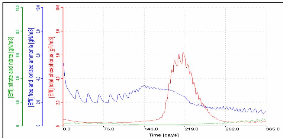
Fig. 7: Simulation results of phosphorus, ammonium and nitrate, in effluent under yearly variation of Wastewater temperature at average influent flowrate
