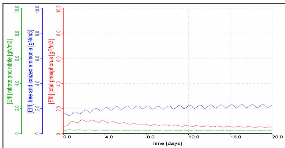
Fig. 4: Simulation results of phosphorus, ammonium nitrate, in effluent under the daily variations of flow and an average wastewater temperature of 16°C
