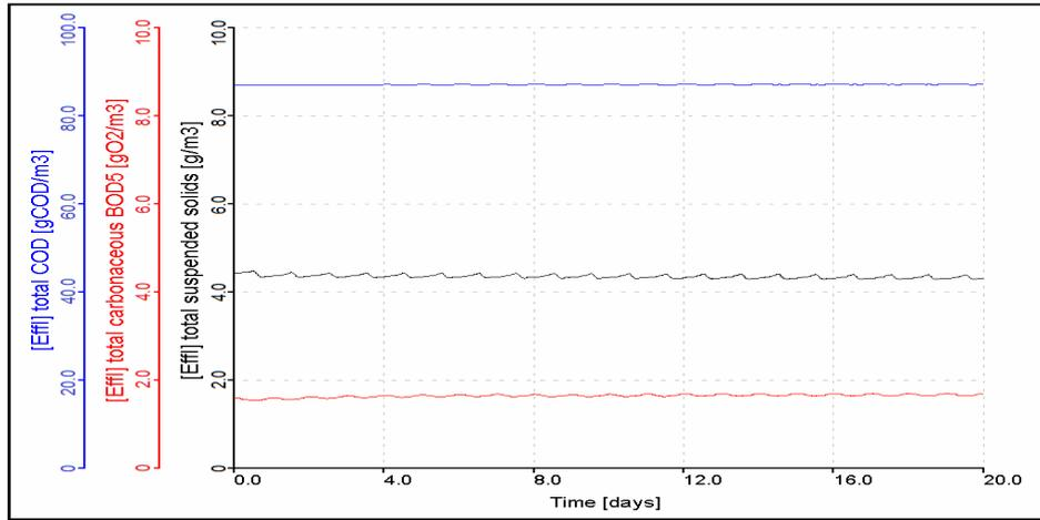
Fig. 5: Simulation results of COD, BOD5 and TSS in effluent under the daily variations of flow and an average wastewater temperature of 16°C.
