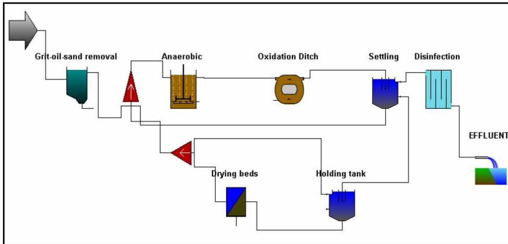
Fig. 2: GPS-X simulation of EBPR for Al-Azeziah WWTP
