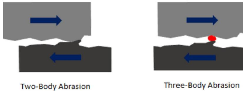
Fig. (5) Main wear mechanisms occurs in drill bit teeth (courtesy of JGS, LSS,2014)
