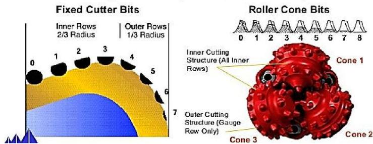
Fig. (2) Bit tooth wear (Reed Hycalog,1999).
