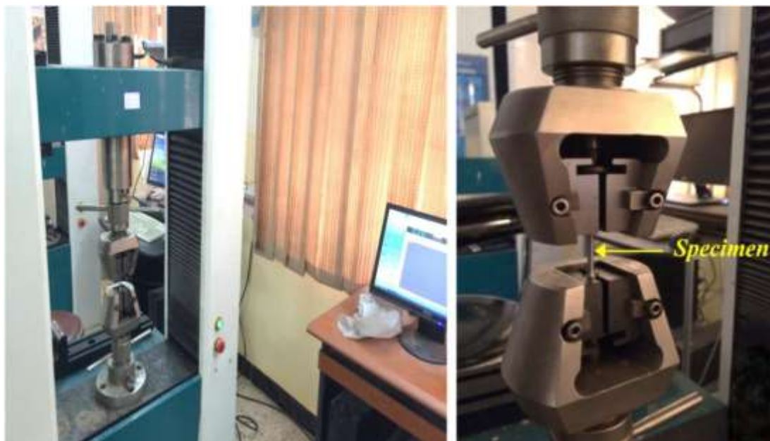
Figure (1): Tensile test device WDW-200E
