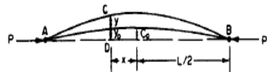
Figure (8): column with initial curvature [14]
