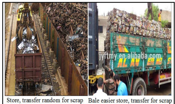
Figure 8: Two methods of store and transfer scrap [15]
