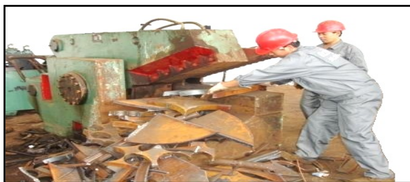
Figure 14: Type of alligator shearing machine [15]
