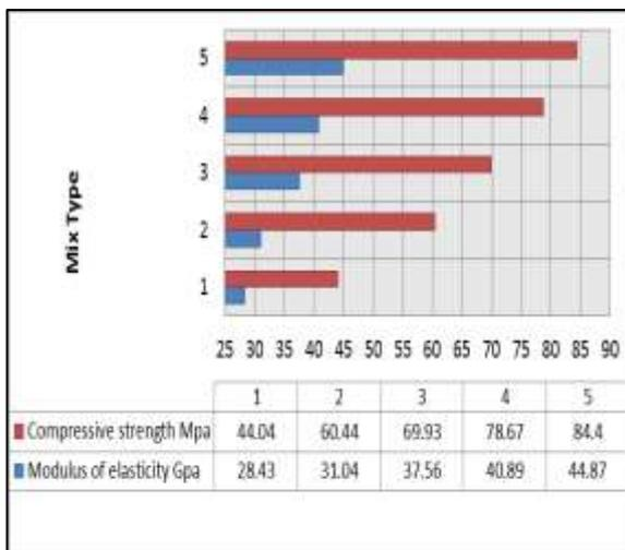
Figure 3: Bar chart of mix type vs. concrete compressive strength and modulus of elasticity at age 28 days
