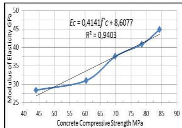
Figure 1: The Relationship between concrete compressive strength and Modulus of Elasticity
