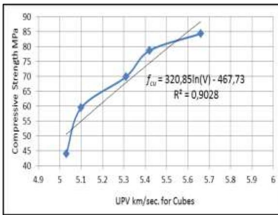
Figure 2: The Relationship between concrete compressive strength and UPV for Cubes
