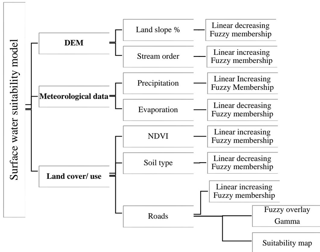
Figure 10: Surface water model utilizing Fuzzy logic overlay
