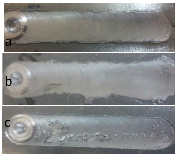
Figure(3): Appearance of welding using cylindrical threaded pin(SCT) at different rotation speed (a) at 450 RPM,(b) at 560 RPM and (c) at 900RPM.
