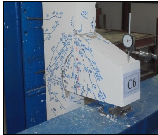
Fig.12-Failure Mode of Specimen C6
