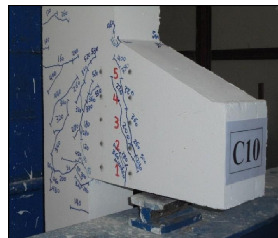
Fig.14-Failure Mode of Specimen C10
