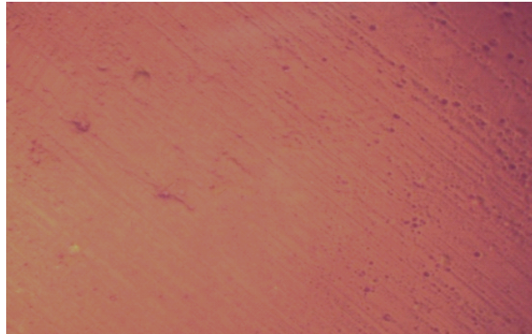
Fig. 9. The microstructure of polystyrene – 30 wt % nano alumina
