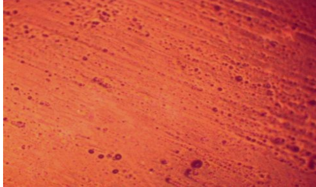
Fig. 7. The microstructure of polystyrene – 10 wt % nano alumina
