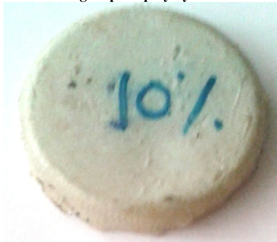
Fig .3. Polystyrene – 10 wt % nano alumina
