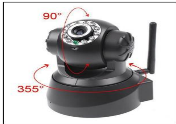
Figure (5) IP camera used in the system.
