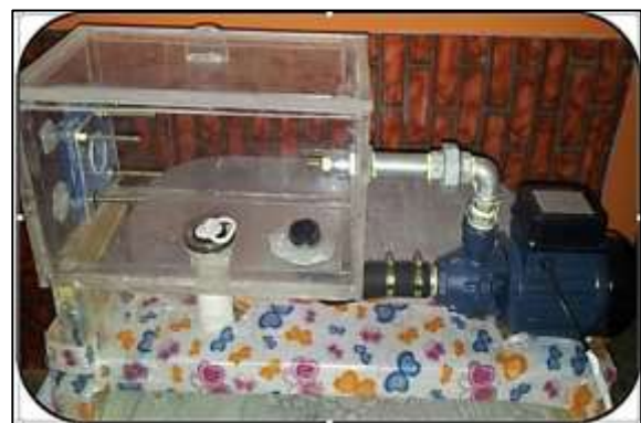
Figure 3: Erosion wear device
