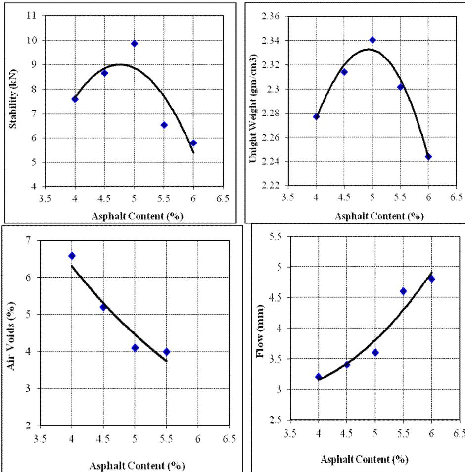
Figure 3. Determination of optimum AC
