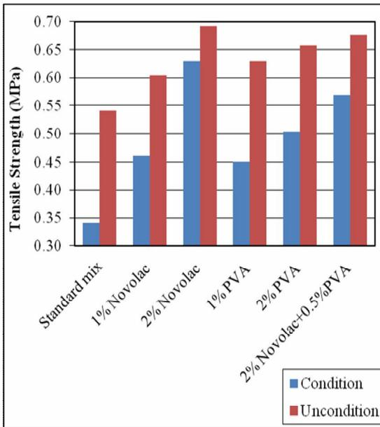
Figure 8. Indirect tensile strength for all mixes
