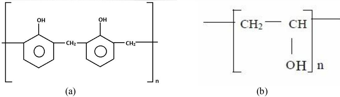
Figure 2. Polymers that are used as additives: (a) Novolac , (b) PVA
