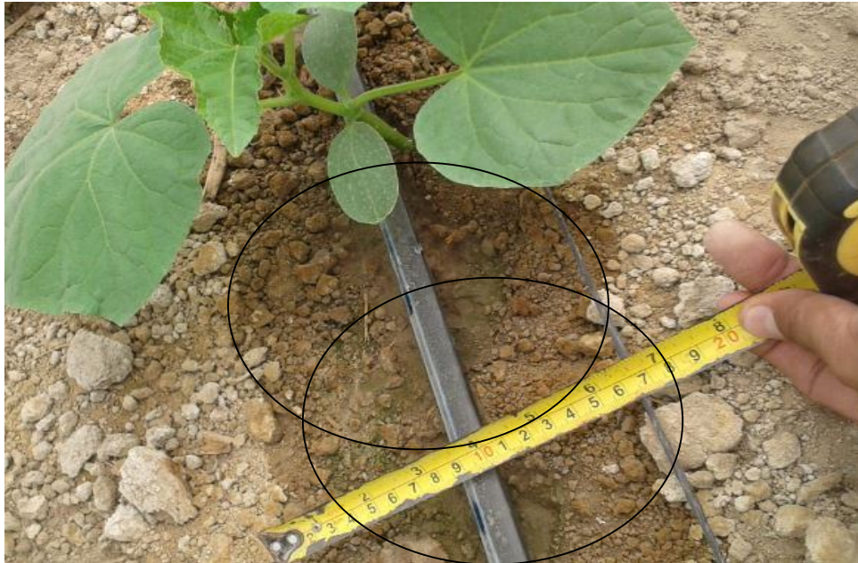
Figure (3) measurement of the wetted area under drip system.
