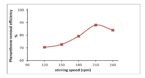
Fig (4): The stirring speed effect on phenanthrene removal efficiency.
