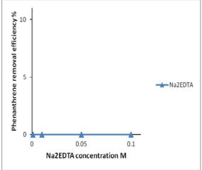
Fig (1): The effect of Na<sub>2</sub>EDTA concentration on phenanthrene removal efficiency.
