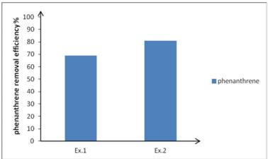
Fig (8): The effect of hydraulic gradient on contaminant removal efficiency in column experiments.
