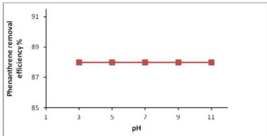
Fig (5): The effect of pH variation on phenanthrene removal efficiency.
