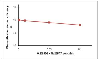
Fig (7): The effect of Na<sub>2</sub>EDTA addition to SDS solution on phenanthrene removal efficiency.
