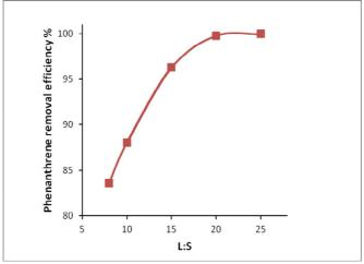
Fig (3): The effect of L/S ratio on phenanthrene removal efficiency.
