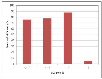
Fig (2): The SDS concentration effect on phenanthrene removal efficiency.
