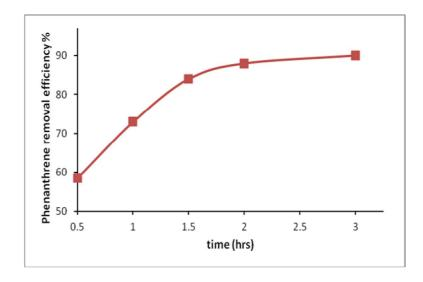
Fig (6): The effect of mixing time on phenanthrene removal efficiency.
