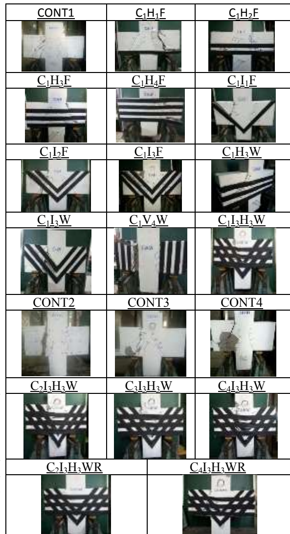
Figure 11: Crack pattern after failure for all corbels specimens
