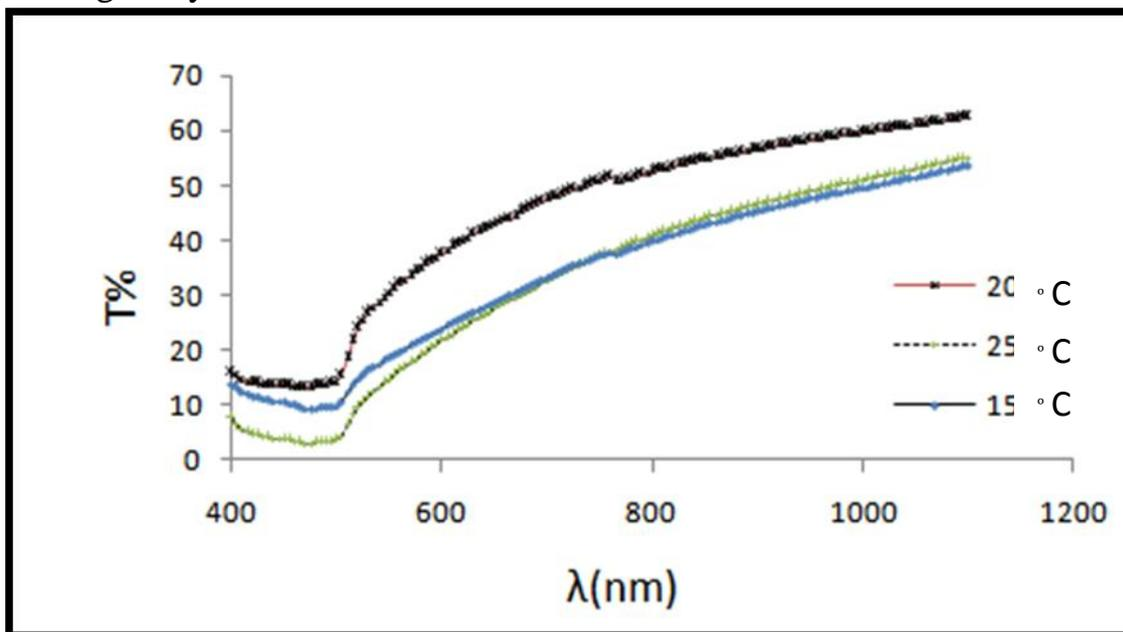
Figure (8): Optical transmission spectrum for  $PbI_2$  films
