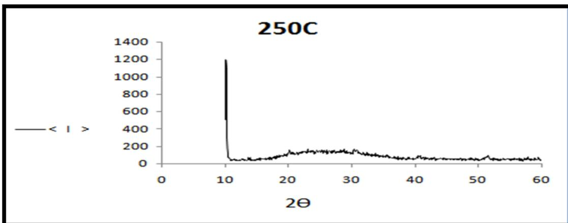
Figure (2) XRD patterns for  $PbI_2$  at different substrate temperature and  $1\mu m$  thickness. a)150° C b)200° C c)250° C
