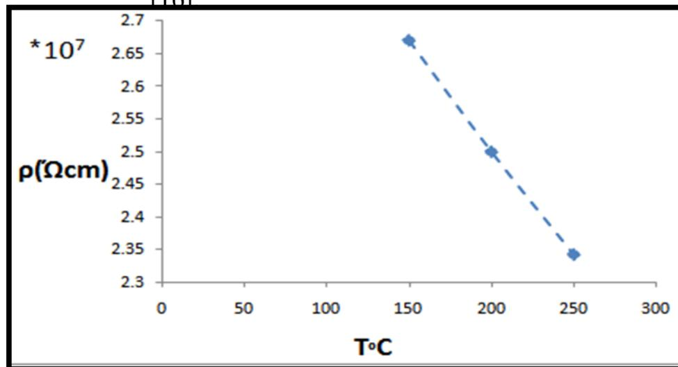
Figure (11): The electrical resistivity as a function of different substrate temperatures 150,200,250° C.
