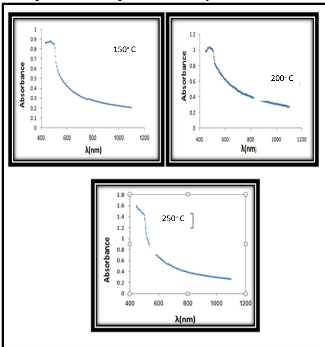
Figure (9): Absorbance vs. wavelength for sample for different substrate temperatures.
