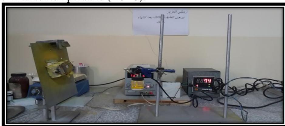
Figure (1): The set up of the spray technique system.
