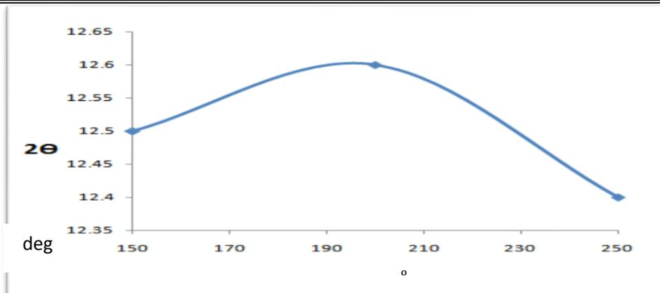
Figure (4) shows the variation of  $2\theta$  as a function of substrate temperature.
