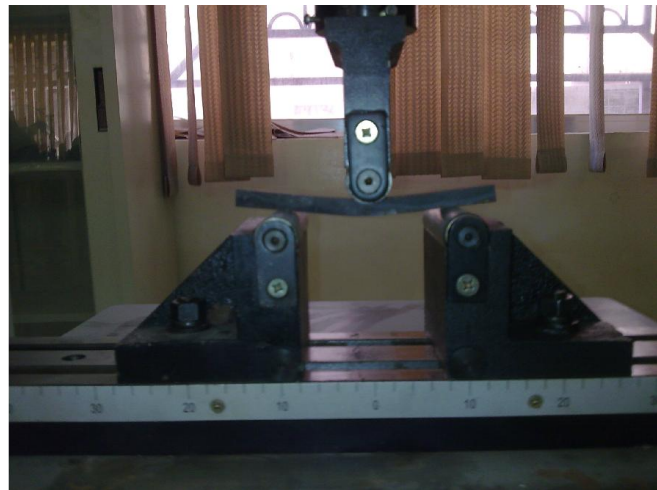
Figure (2) Bending test apparatus
