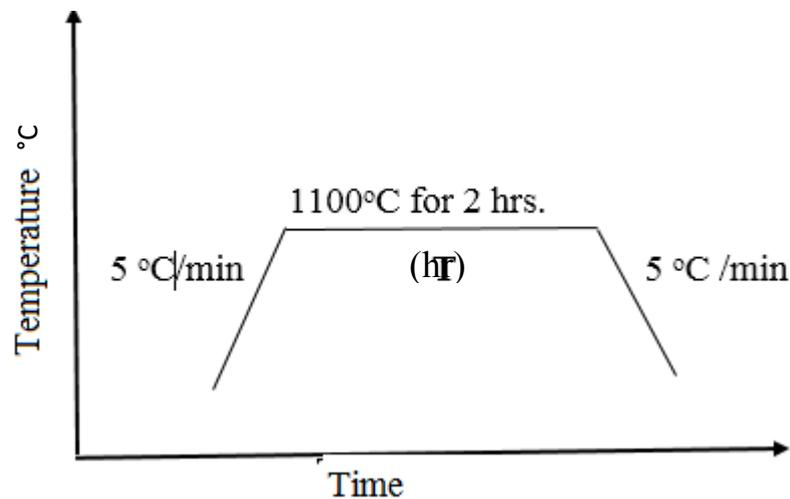
Figure (1): Single heating cycle of the applied sintering process.
