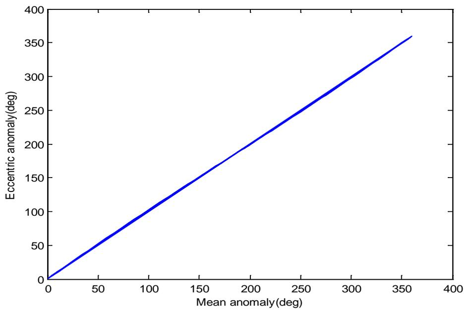
Fig(6). The eccentric anomaly (deg) against mean anomaly (deg) for quasi-circular orbit
