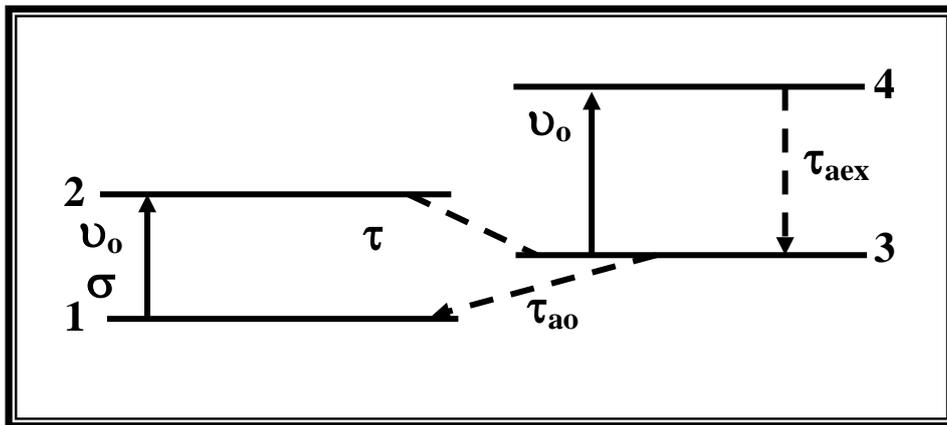
Fig.1 : The absorption dynamic of the saturable absorber [24] .
