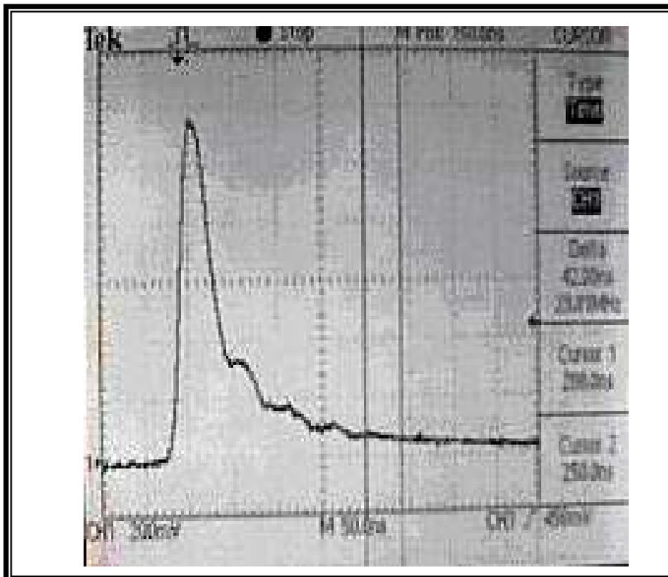
Fig.4 The Q-switched laser pulse
