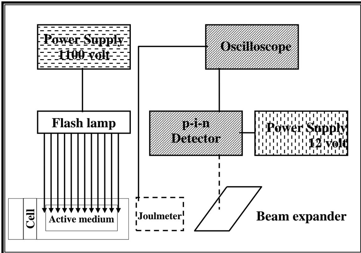
Fig.2 : The experimental setup of a passively Q- switched Nd:YAG laser system.
