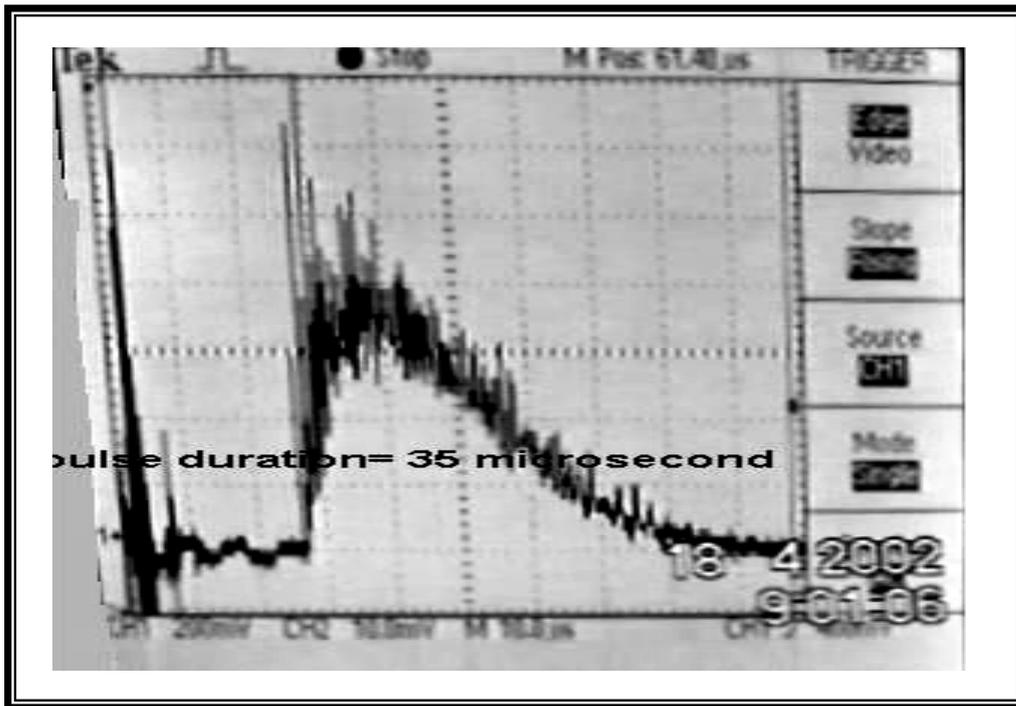
Fig.3: The free-running pulse of Nd:YAG laser
