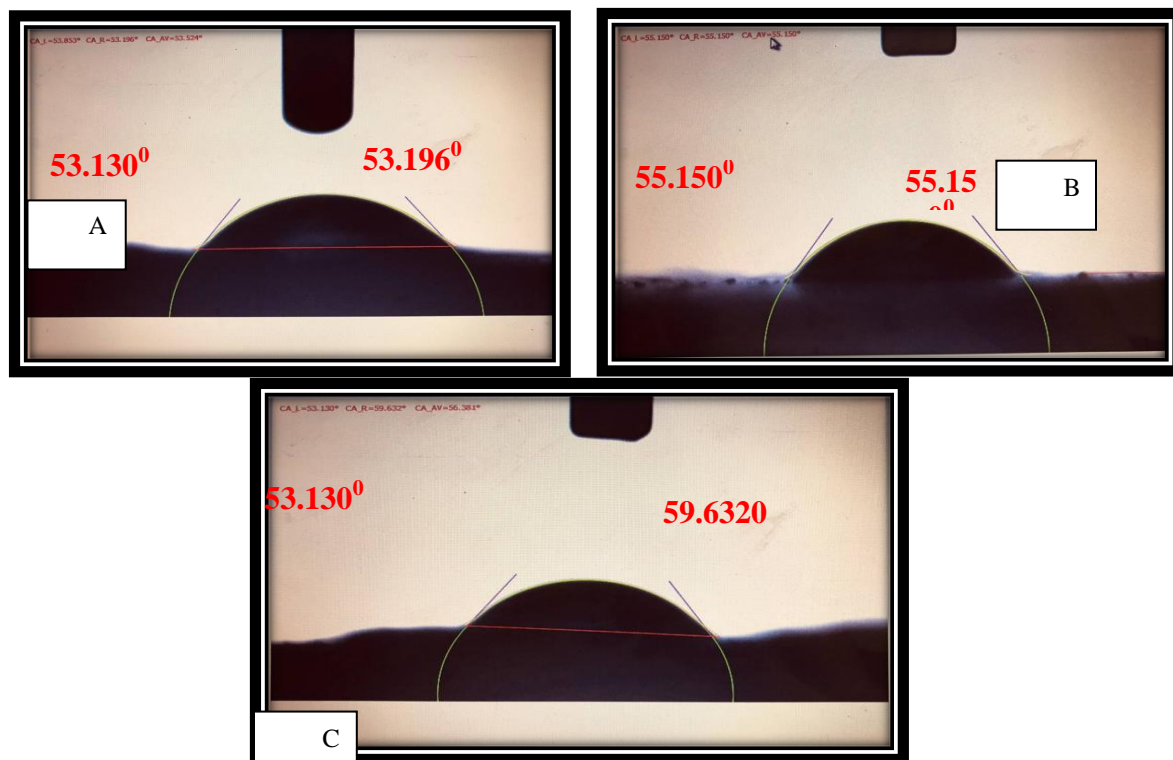
Figure 5 : static contact angles of wettability test. A, control specimen B, 0.25% MMTNPs specimen C, 0.5% MMTNPs specimen.
