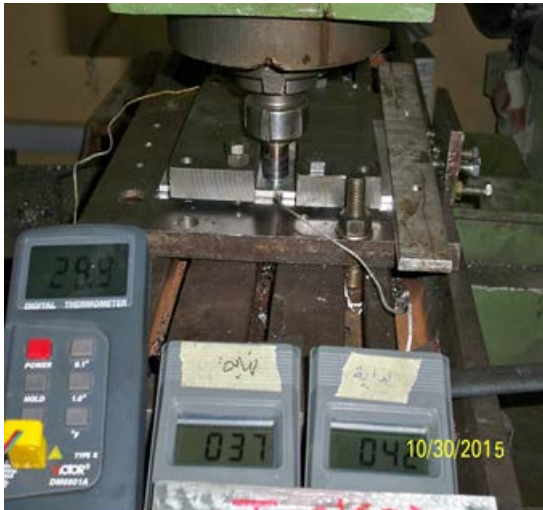
Figure (5): Temperature recorder by thermocouple position on work-piece
