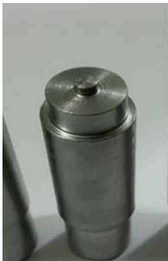
Figure (2): schematic diagram explain the shape of the welding tool.
