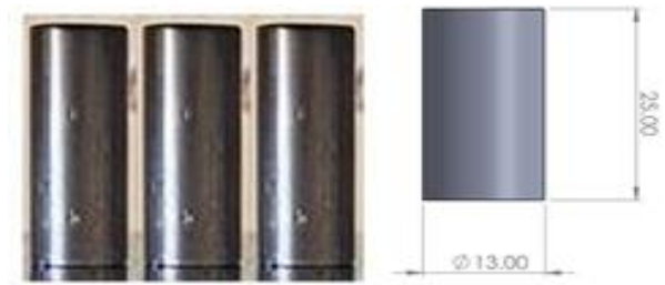
Figure 5. Compression specimen for Ti-13Nb-13Zr
