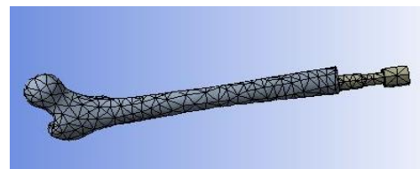
Figure 11. Meshed model with ten-node tetrahedral elements
