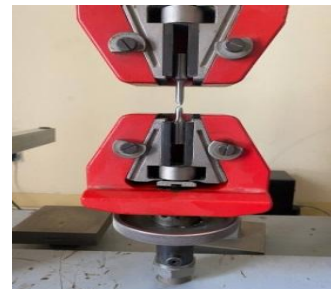
Figure 2. Tensile test setup
