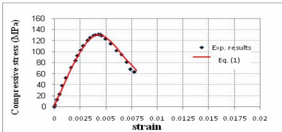
Fig.(6) Compressive stress-strain curves of RPC mix (MSF10)
