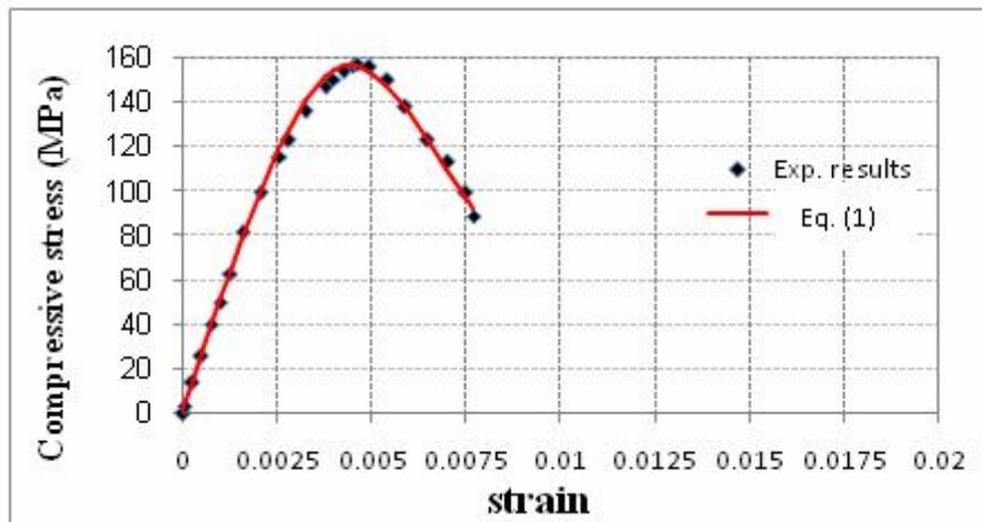
Fig.(8) Compressive stress-strain curves of RPC mix (MSF30)
