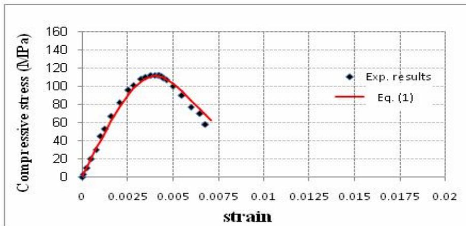
Fig.(5) Compressive stress-strain curves of RPC mix (MSF0)
