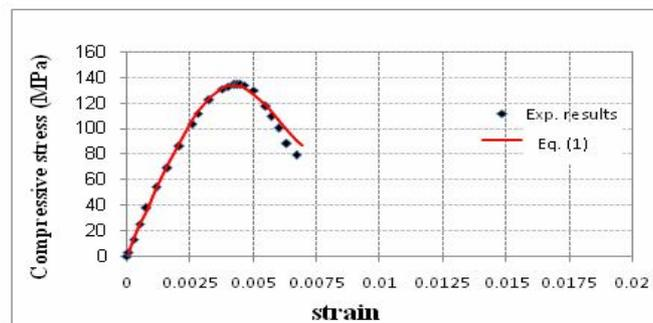
**Fig.(4) Compressive stress-strain curves of RPC mix (MSP-P)**
