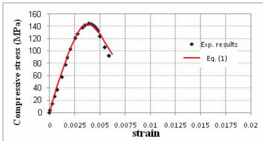
Fig.(10) Compressive stress-strain curves of RPC mix (MFR1)
