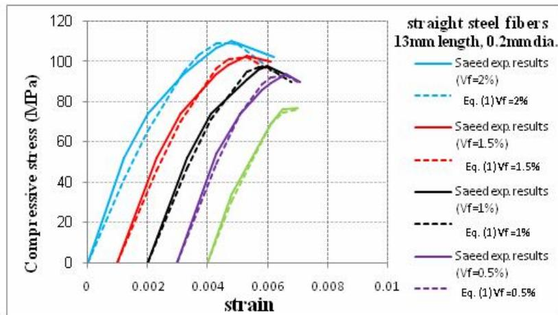
Fig.(13):A Comparison between Saeed 2010 experimental compressive stress-strain curves and the proposed model (Equation 1)
