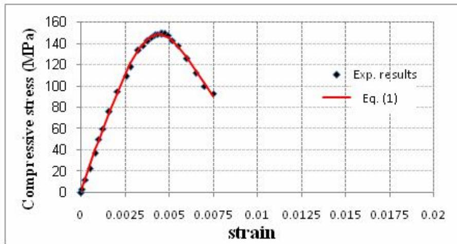
Fig.(11) Compressive stress-strain curves of RPC mix (MFR2)
