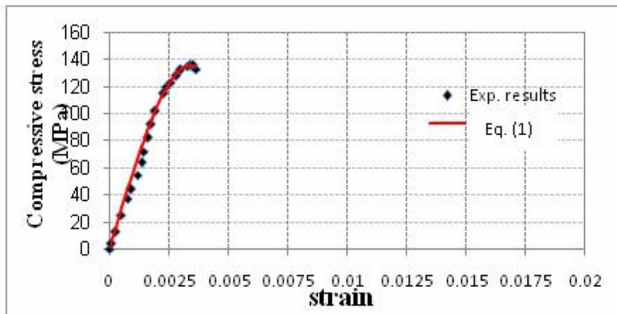
Fig.(9) Compressive stress-strain curves of RPC mix (MFR0)
