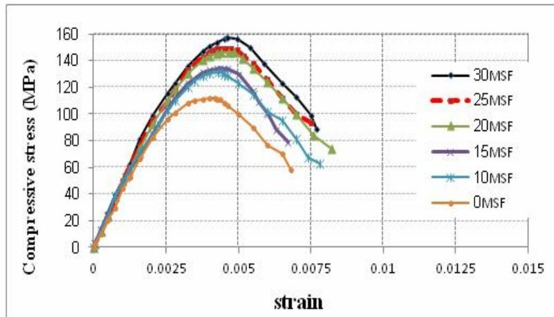
**Fig. (2): Effect of silica fume content (SF) on the compressive stress-strain relationship of RPC**
