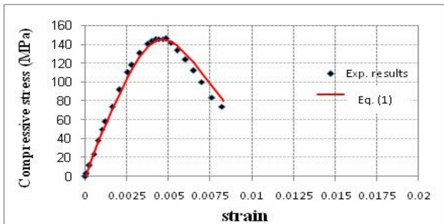
Fig.(7) Compressive stress-strain curves of RPC mix (MSF20)
