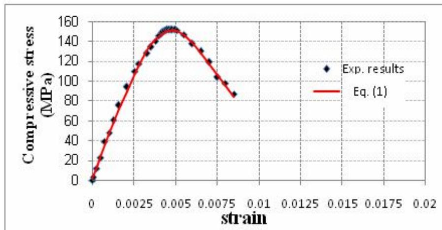
Fig.(12) Compressive stress-strain curves of RPC mix (MFR3)
