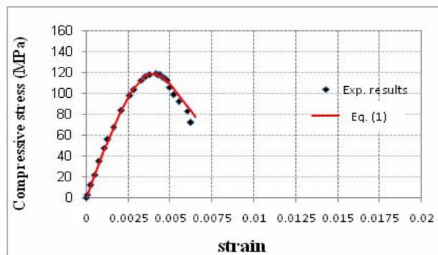
**Fig.(3): Compressive stress-strain curves of RPC mix (MSP-N)**
