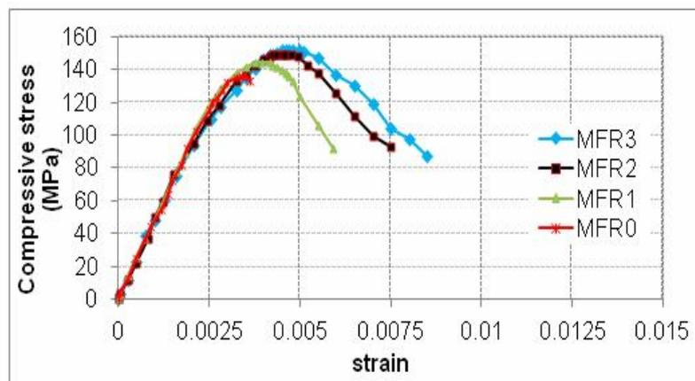
**Fig.(1) :Effect of steel fibers volume fraction on the compressive stress-strain relationship of RPC**
