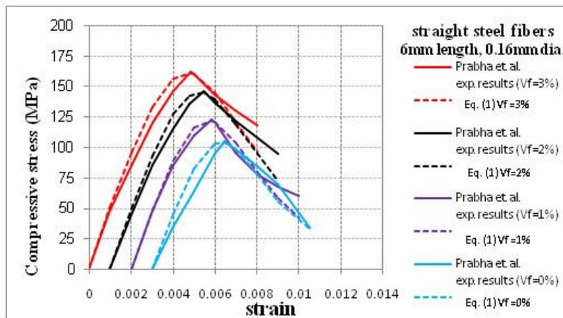
Fig.(14):A Comparison between Prabha et al. 2010 experimental compressive stress-strain curves and the proposed model (Equation 1)
