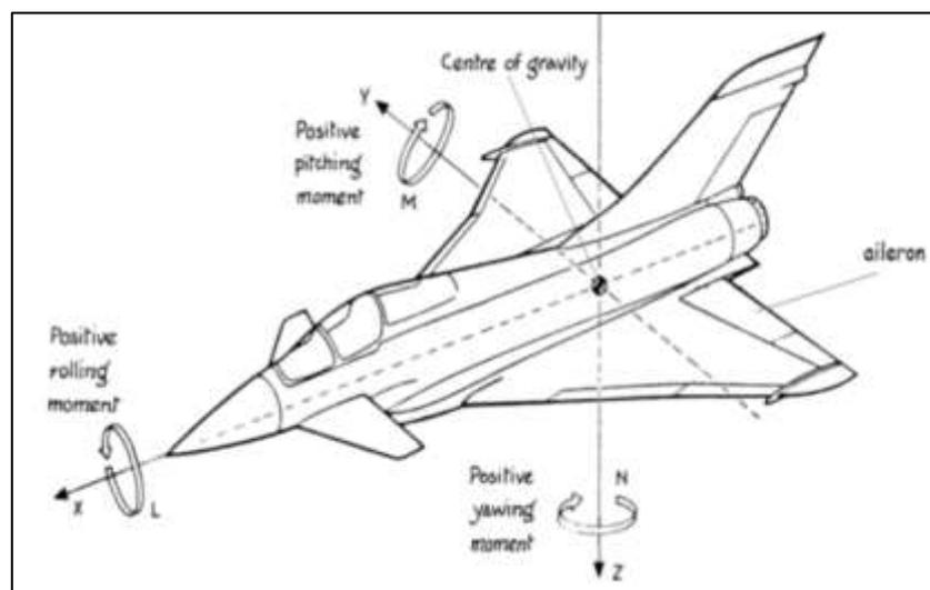
Figure 1: Basic sketch of delta wing aircraft [2]
