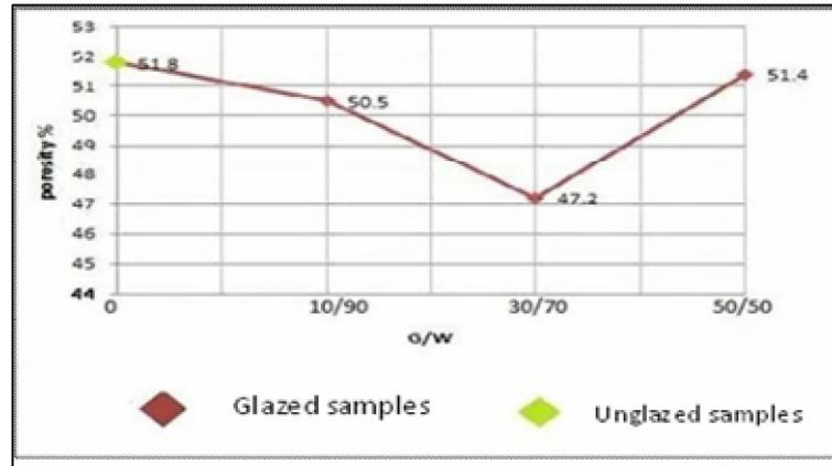
Fig.(1-2):Porosity of A<sub>4</sub>-glazed samples as a function of G/W
