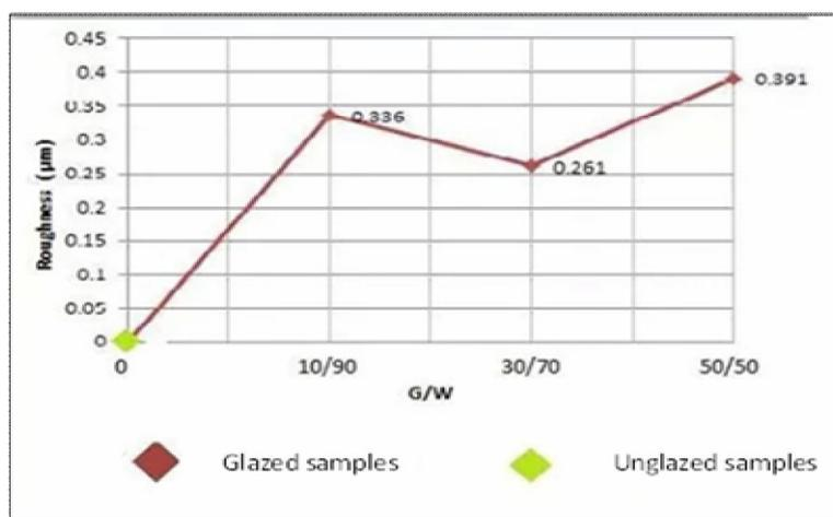
Fig.(1-8): Surface roughness of  $A_5$ -glazed samples as a function of G/W mixing ratio
