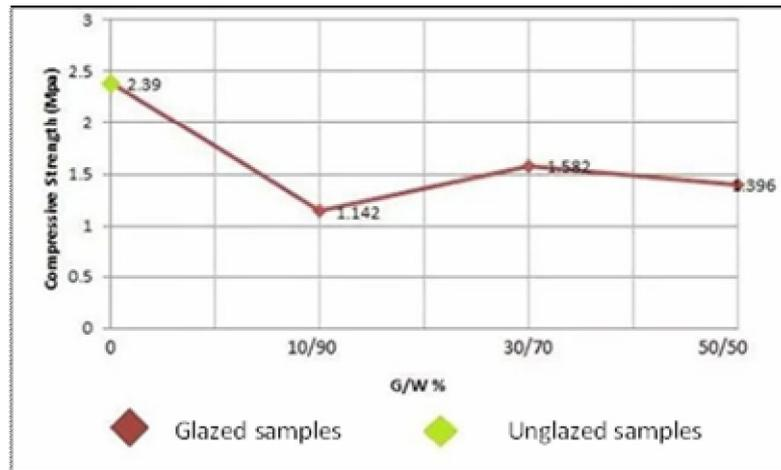
Fig.(1-9): compressive strength of  $A_4$ -glazed samples as a function of G/W
