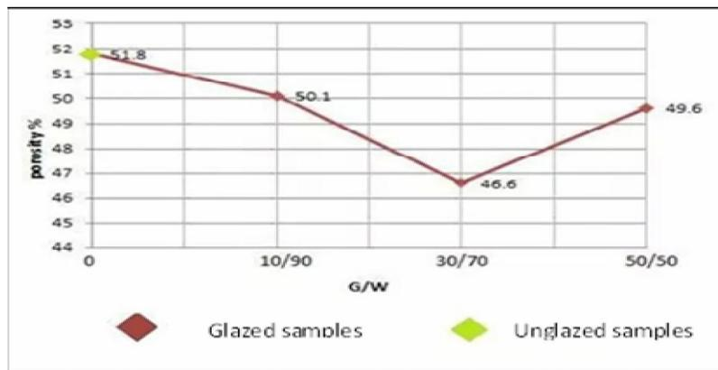
Fig.(1-3):Porosity of A<sub>5</sub>-glazed samples as a function of G/W mixing
