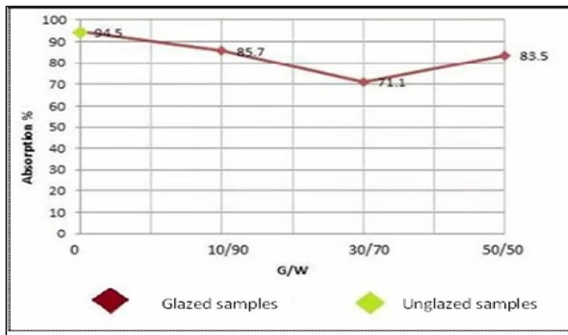
Fig.(1-4):Water absorption of A<sub>4</sub>-glazed samples as a function of G/W mixing ratio
