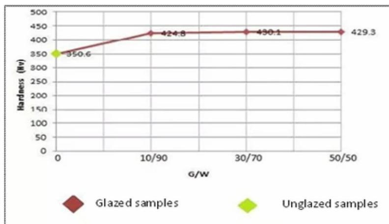
Fig.(1-11): Vickers hardness of  $A_4$ -glazed samples as a function of G/W
