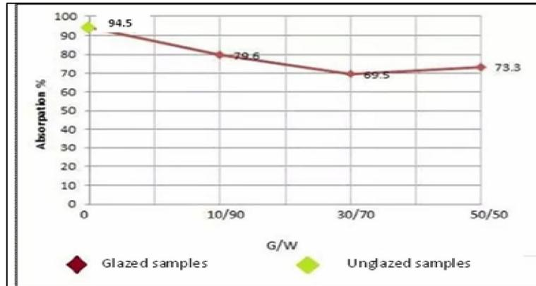
Fig.(1-5): Water absorption of A<sub>5</sub>-glazed samples as a function of G/W
