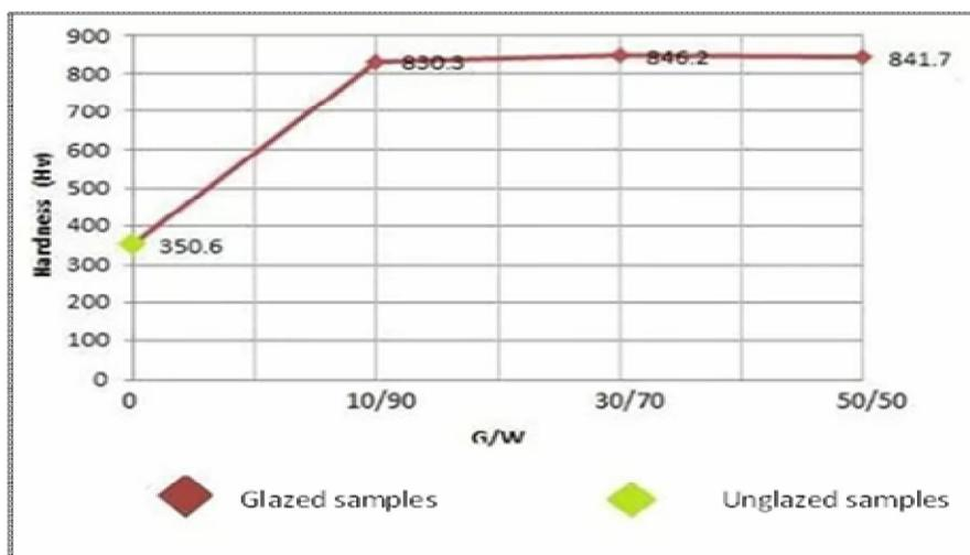
Fig.(1-12): Vickers hardness of A<sub>5</sub>-glazed samples as a function of G/W mixing ratio
