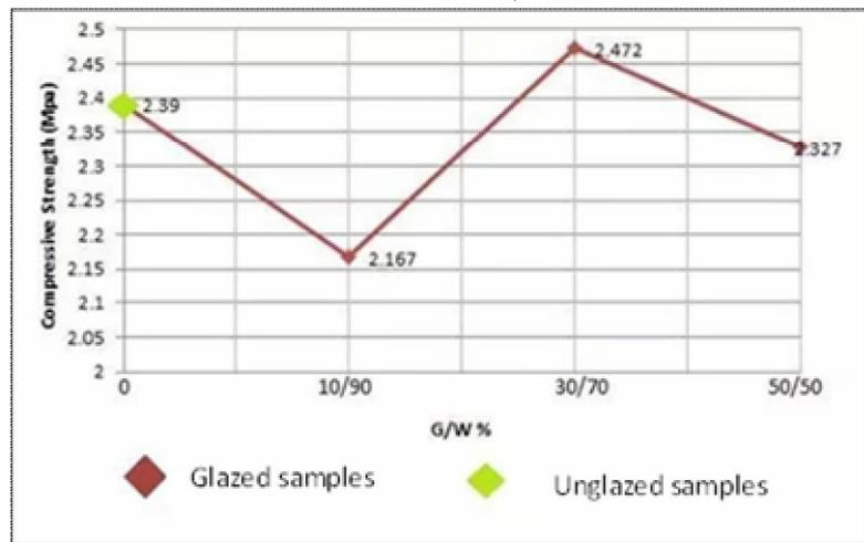
Fig.(1-10): compressive strength of  $A_5$ -glazed samples as a function of
