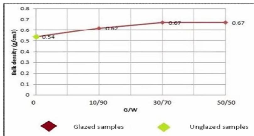
Fig.(1-7): Bulk density of A<sub>5</sub> – glazed samples as a function of G/W
