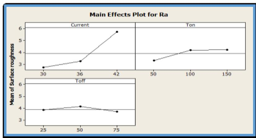
Figure 10: Mean effects plot for Surface roughness
