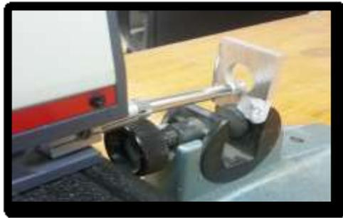
Figure 6: Pocket Surf holder for the proposed work
