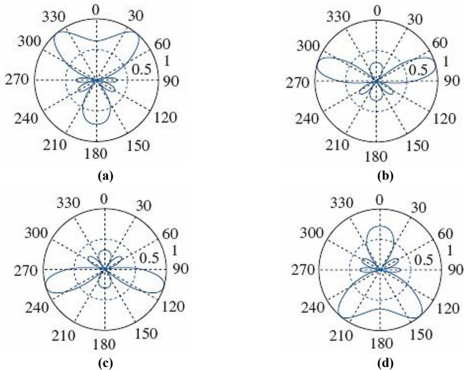
Fig. 5. Four examples of the obtained radiation pattern of 8-elements PAA. (a) Beam no. 4 with ( $\theta = 39.38^\circ$ ), (b) Beam no. 7 with ( $\theta = 73.13^\circ$ ), (c) Beam no. 10 with ( $\theta = 106.88^\circ$ ), (d) Beam no. 13 with ( $\theta = 140.63^\circ$ ).
