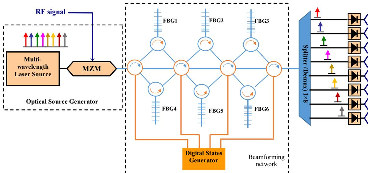
Fig. 3. Proposed phased array antenna system
