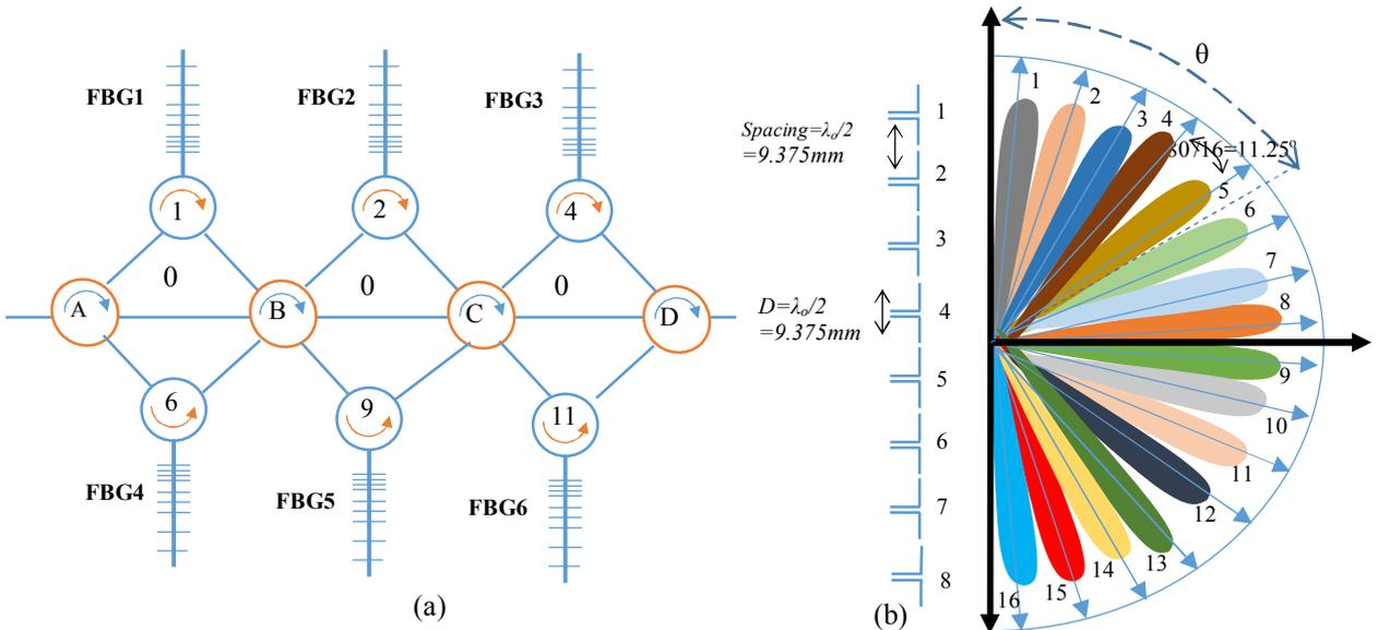
Fig. 4. (a) The proposed delay lines based on Fiber Bragg Gratings (FBG), (b) Schematic radiation pattern representation of the proposed phased-array antenna.
