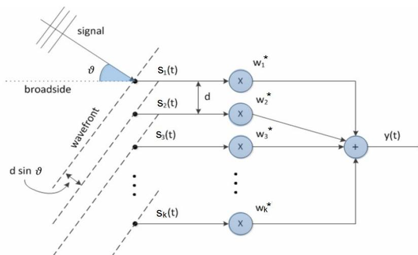
Fig 1. Uniform linear array with a beam-steering network (Liu and Weiss 2010)
