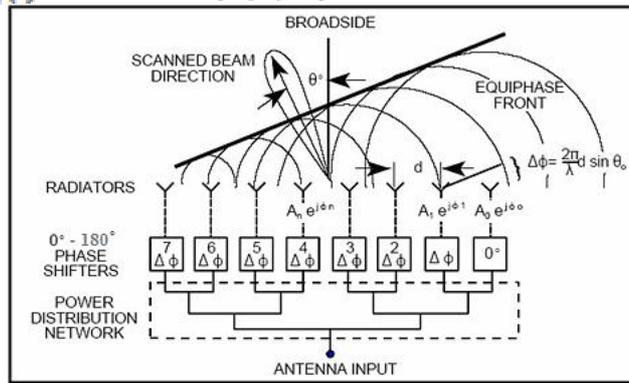
Fig. 2. Typical phased-array antenna architecture (Vidal et. al. 2012).
