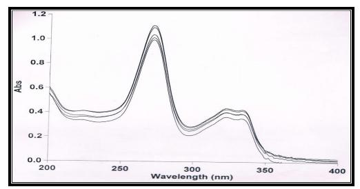
Fig (3b) UV.spectrum of chitosan-ciprofloxacin release in pH1.1 at 37°C at271 nm
