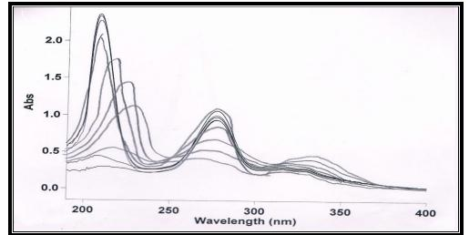
Fig (3a) UV.spectrum of chitosan-ciprofloxacin release in pH7.4 at 37  $^\circ C$  at  $\lambda max210$  and 278nm
