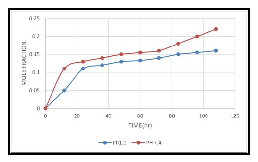
Fig (4) controlled ciprofloxacin release from a mide prodrug chitosan in pH7.4 and 1.1 at  $37^\circ C$  in 271nm
