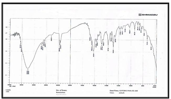
(Fig5) FTIR spectrum of Cipro chitosan prodrug polymer
