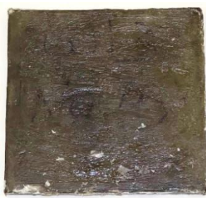
Figure 3. Composite plate from the previous stage (20 X 20) cm
