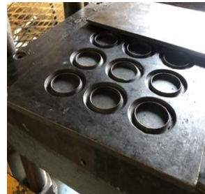
Figure 5. Hardness specimen mold.
