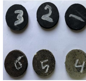
Figure 7. The hardness test specimen (d:12, h:24) mm.
