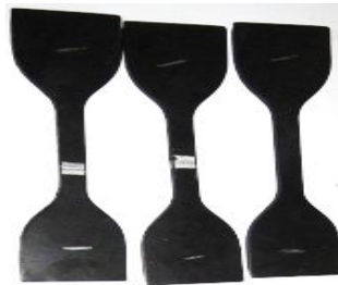
Figure 12. Dumbbell shape specimen. 2 mm thickness and 165 mm effective length.
