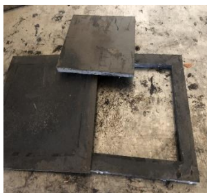
Figure 2. Hard composite mold, (20 X 20) cm
