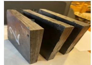
Figure 17. Vulcanized plates with rubber recipe
