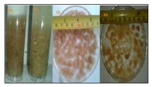
Figure 3: Photo of granules of RR and RD reactors
