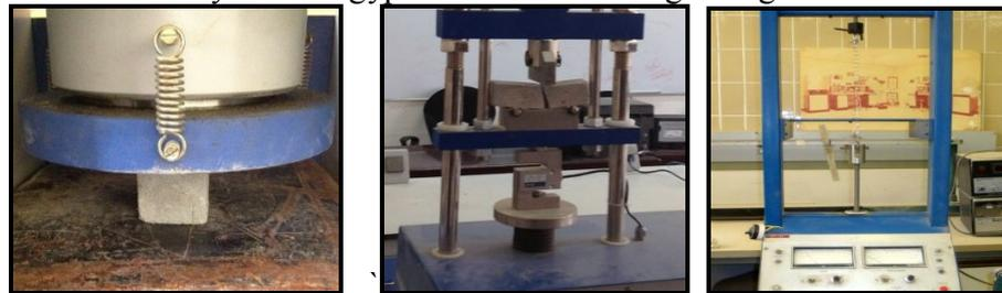
d- Ferrocement components tests (cement mortar and fabricated wire mesh)
