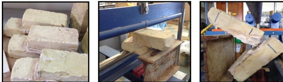
c- Clay bricks - gypsum mortar bonding strength test
