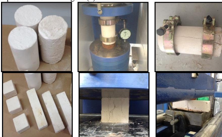
a- Gypsum mortar tests
