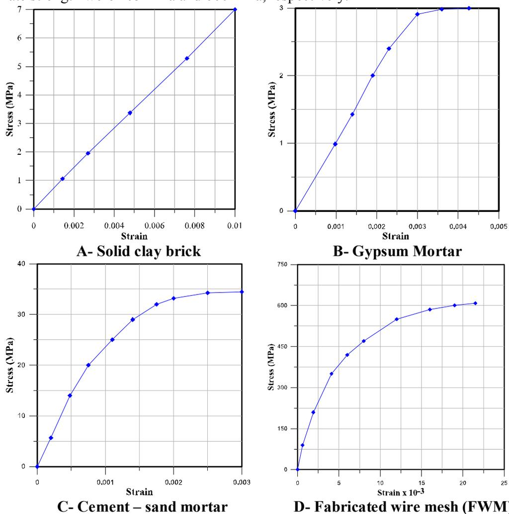
Figure (1) Stress –strain relationships of used materials in brickwork arches Fabrication
