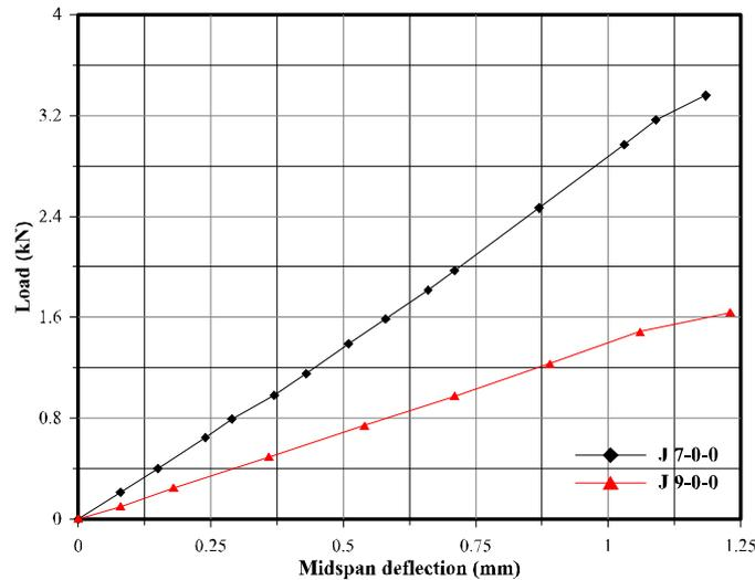
**Figure (4) Panel width effect upon strength and variation of mid-span deflection with applied load for jack arch specimens without camber or ferrocement layer**
