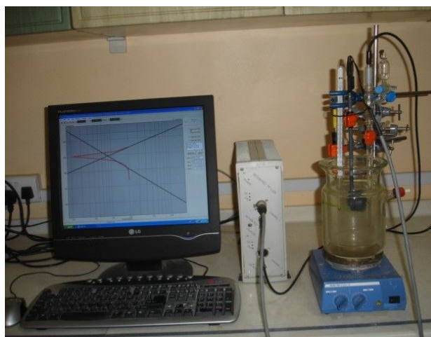
Fig 2. The electrochemical corrosion unit.
