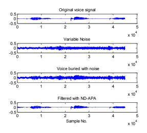
Figure 10: Processed voice waveform using ND-APA.
