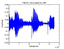
Figure 11: Voice waveform processed by LMS.
