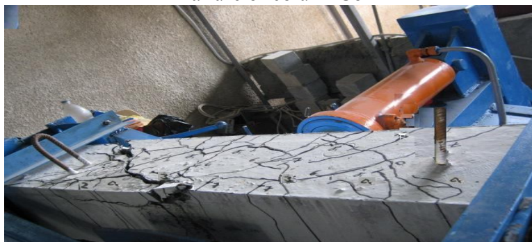
Failure of columnC7
