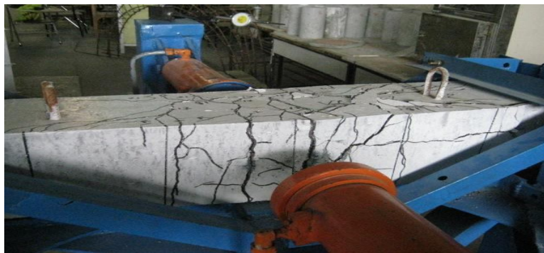
Failure of columnC8
