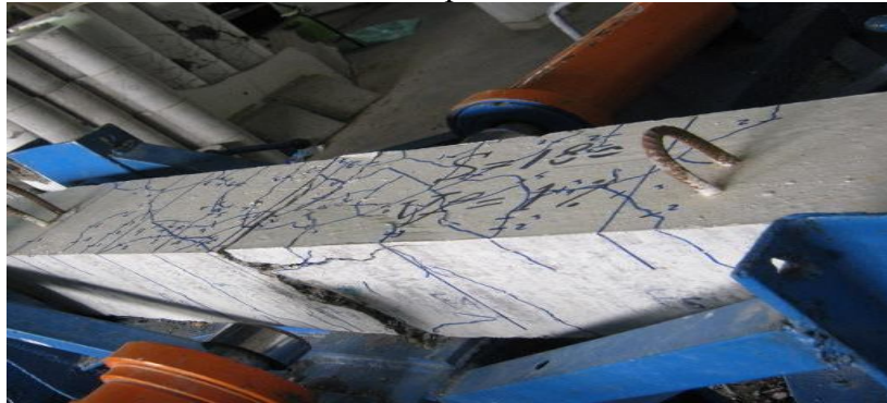
Failure of specimen C10
