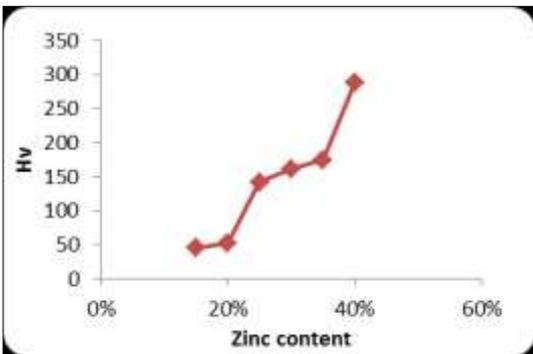
Figure 17: Vickers micro hardness curves for alloys
