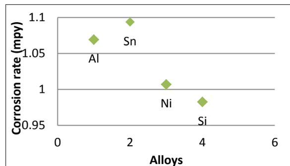
Figure25: Corrosion rate (mpy) of the alloy in seawater media
