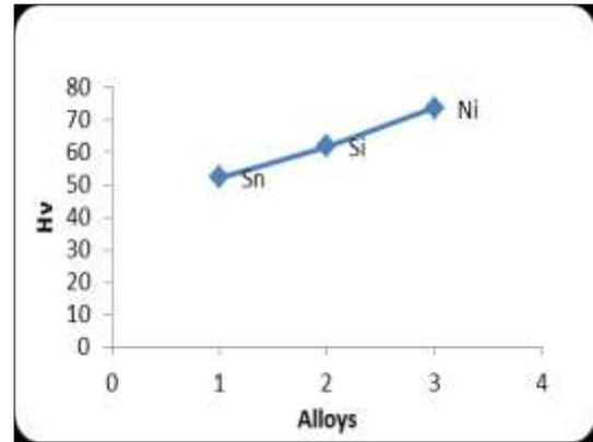
Figure18: Vickers micro hardness curves for alloys without additives
