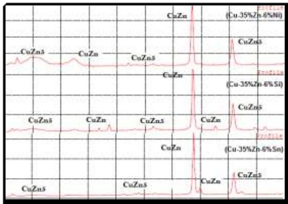
Figure 2: XRD pattern for (Cu-35%Zn with Si, Sn and Ni) that sintered at 650°C for 4 hr
