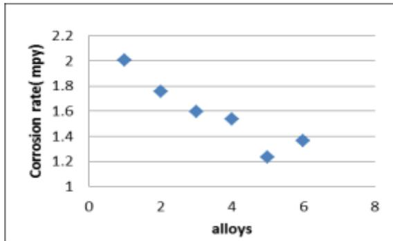
Figure 22: Corrosion rate (mpy) of the Alloys in NaOH
