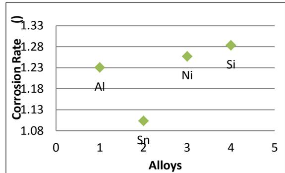
Figure23: Corrosion rate (mpy) of the Alloys with additives in NaOH
