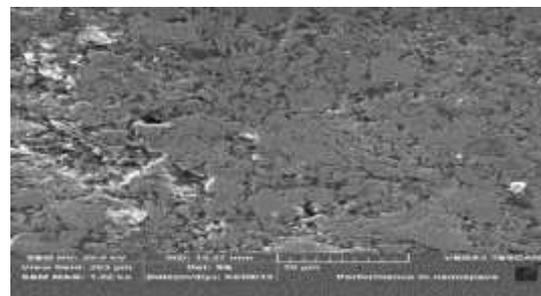
Figure 15: SEM of sample (Cu-35%Zn-6%Si alloy)
