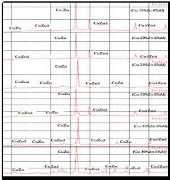
Figure 1: XRD pattern for (Cu-Zn-Al) samples that sintered at 650°C for 4 hr
