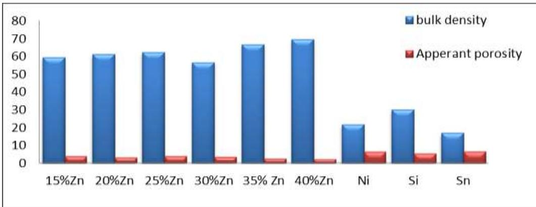
Figure19: Apparent porosity and bulk density results for alloys and alloys with additives
