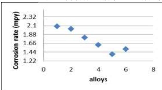
Figure 20: Corrosion rate (mpy) of the Alloys in HCl
