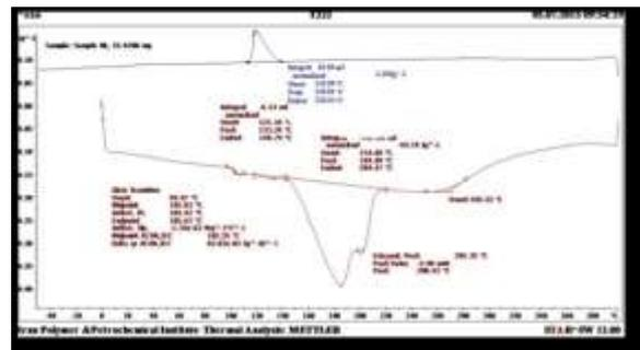
**Figure 6: Transformation temperature of alloy (Cu-30wt%Zn-6wt%Al)**
