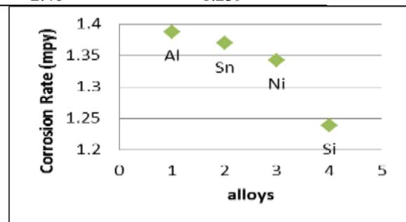
Figure 21: Corrosion rate (mpy) of the Alloys with additives elements in HCl media
