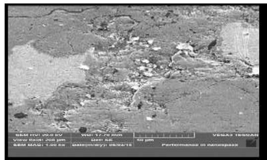
Figure 14: SEM of sample (Cu-35%Zn-6%Ni alloy)
