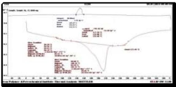
**Figure5: Transformation temperature of alloy (Cu-25wt%Zn-6wt%Al)**
