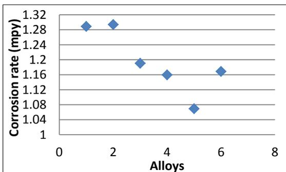
Figure 24: Corrosion rate (mpy) of the sample in seawater Media
