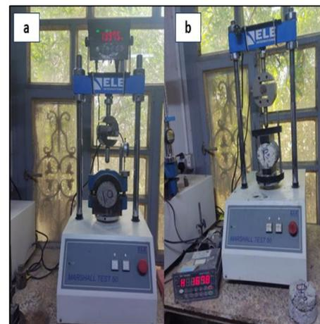
**Figure 12.** Methods of testing setup: (a) Marshall stability device, and (b) ITS device.
