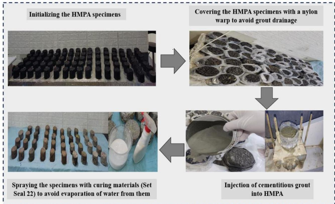
**Figure 11.** Steps of formulation of SFP specimens.
