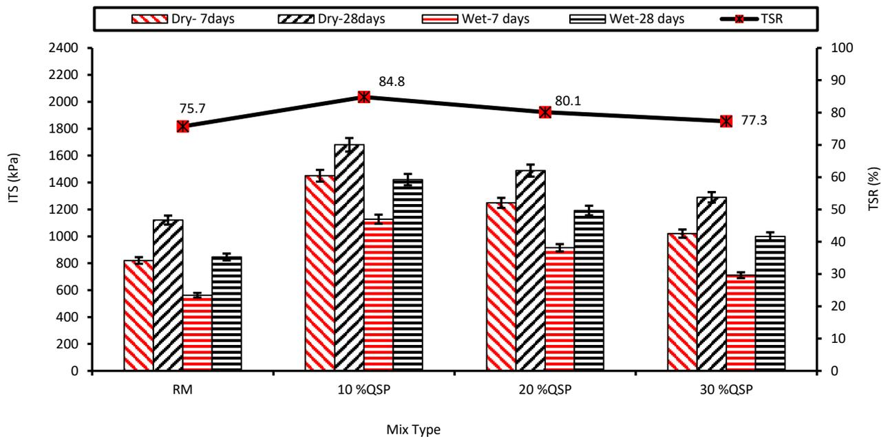
Figure 16. The results of ITS and TSR for conventional and modified SFP mixtures with QSP at 7 and 28 days of curing
