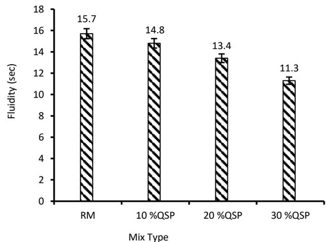
Figure 13. Fluidity results of conventional and modified cementitious grout with QSP.3.
