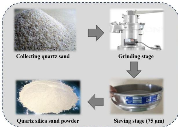
Figure 5. Schematic of QSP preparation.
