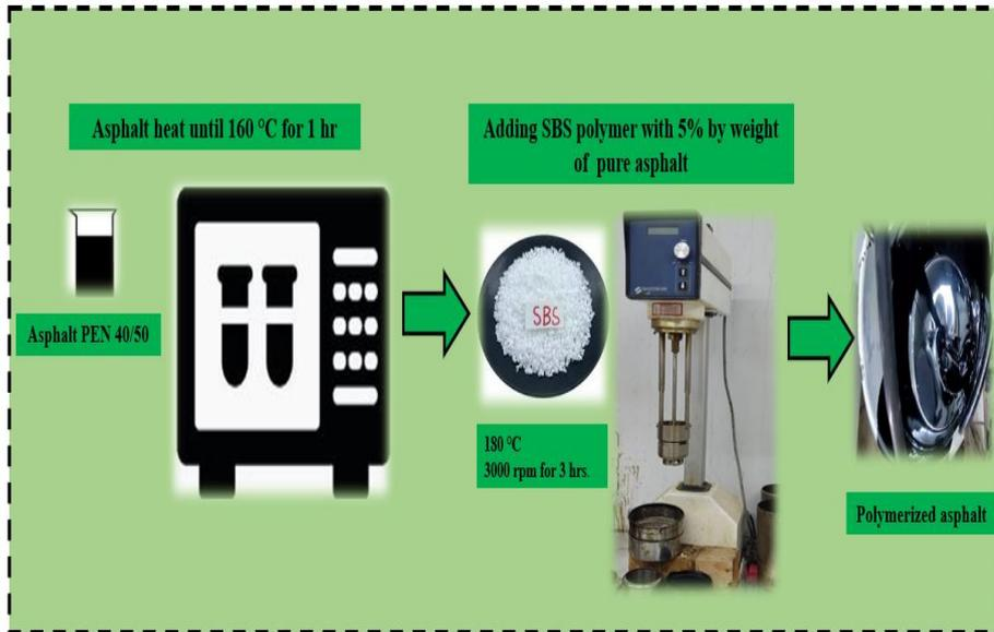
Figure 7. Schematic of the preparation of SBS-modified asphalt in this study.
