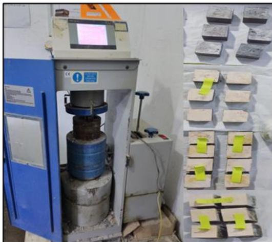
**Figure 10.** The compressive strength device with its specimens.
