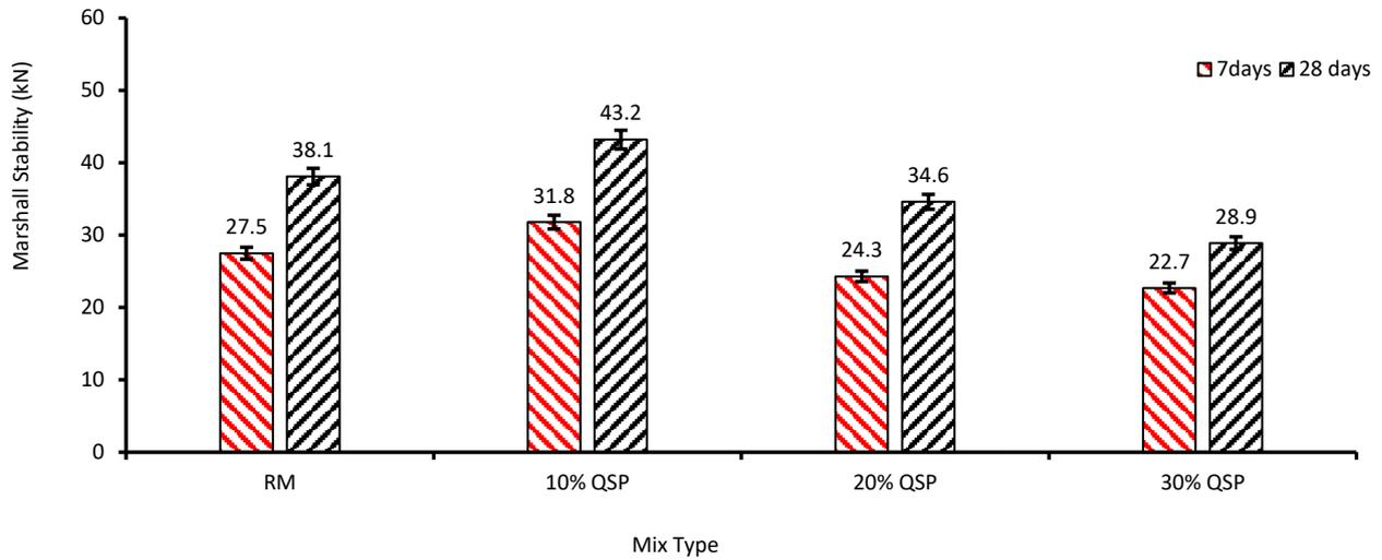
Figure 15. The Marshall stability findings for conventional and modified SFP specimens with various content of QSP at 7 and 28 days of curing.
