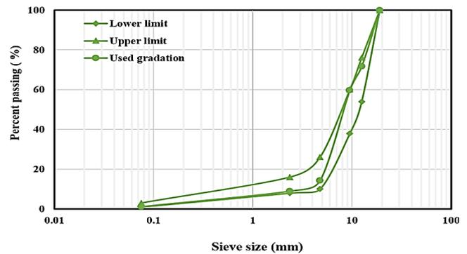
Figure 6. The open-graded HMPA according to ASTM D7064 [34]
