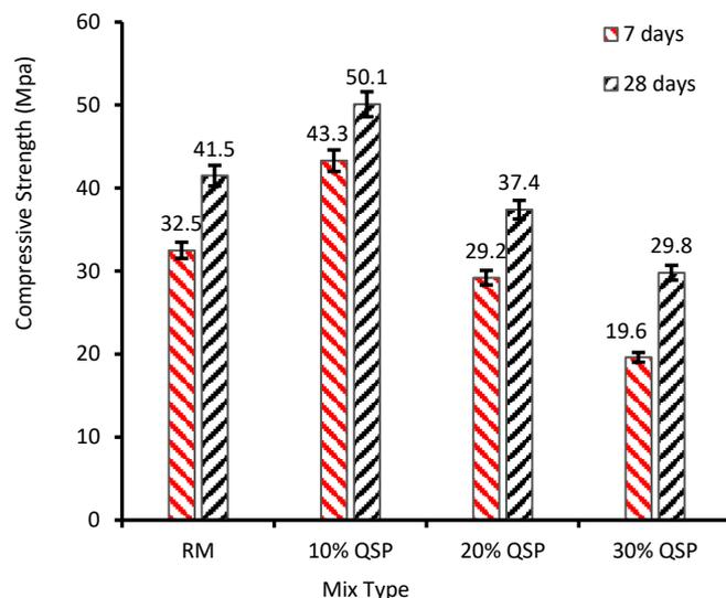
**Figure 14.** Compressive strength results for conventional and modified cementitious grout with QSP at 7 and 28 days of curing.
