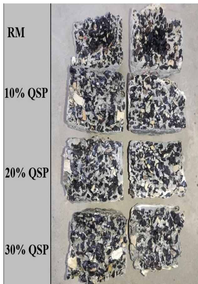
**Figure 17.** The difference between control and QSP-modified SFP mixtures after the ITS test.
