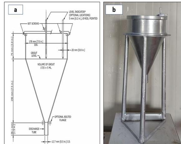
Figure 8. Flow cone test setup : (a) flow cone device measurement schematic [42], and (b) ASTM flow cone.
