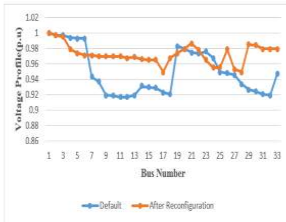
Figure 7: Voltage profile for 33-bus before and after re-configuration network analysis
