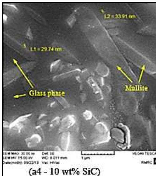
Figure 2: SEM images for Nano β –SiC specimens.
