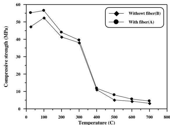
Figure (1) Compressive strength- temperature relationship for fibrous and non fibrous concrete.
