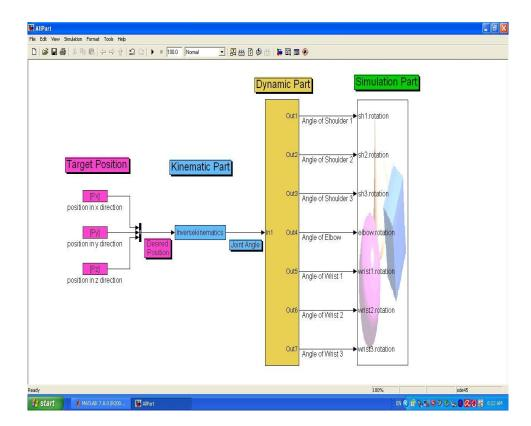
Figure . 4. The Simulink model for A Human Arm
