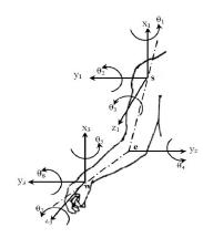
Figure.1. Kinematic chain of human arm
